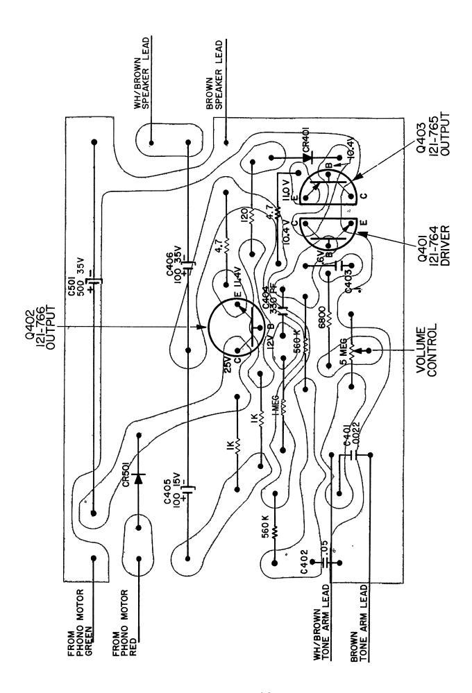
3AT20 CHASSIS WIRING AND COMPONENTS AS VIEWED FROM FOIL SIDE — LATER PRODUCTION
