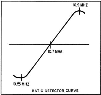
Because of the wide band pass required in the multiplex FM receiver, it is desirable to use an FM signal generator having a deviation of at least 200 KHz with a sweep rate of 60 Hertz, as well as arm oscilloscope. During the IF and ratio detector alignment it is not only necessary to obtain maximum gain, but also ex tremely important to maintain symmetry.
