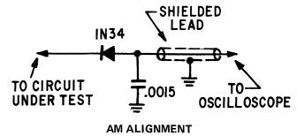
C. A V.T.V.M. on low AC scale connected across the speaker voice coil output terminals (either left or right channel), will be satisfactory for all AM, IF and RF adjustments.
