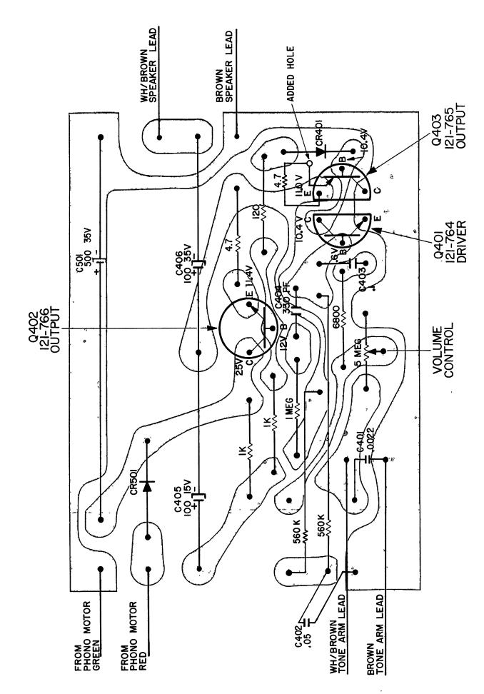
3AT20 - CHASSIS WIRING AND COMPONENTS AS VIEWED FROM FOIL SIDE EARLY PRODUCTION
